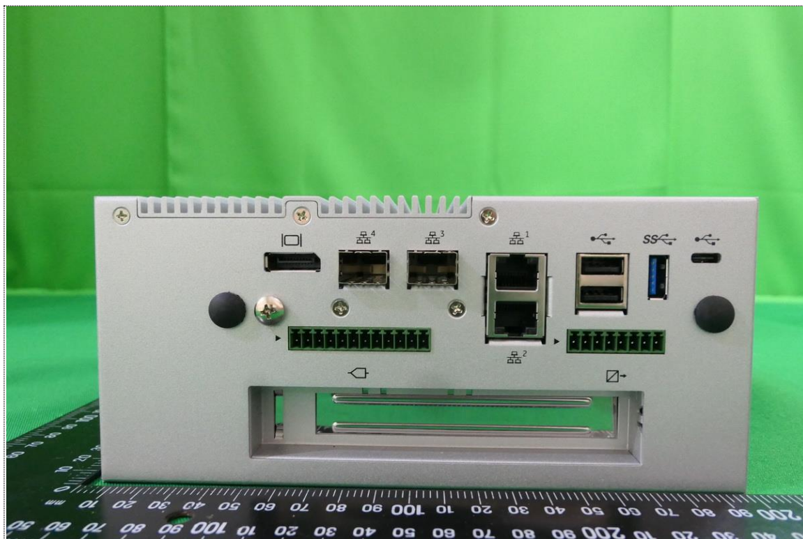
View of I/O Port-1
