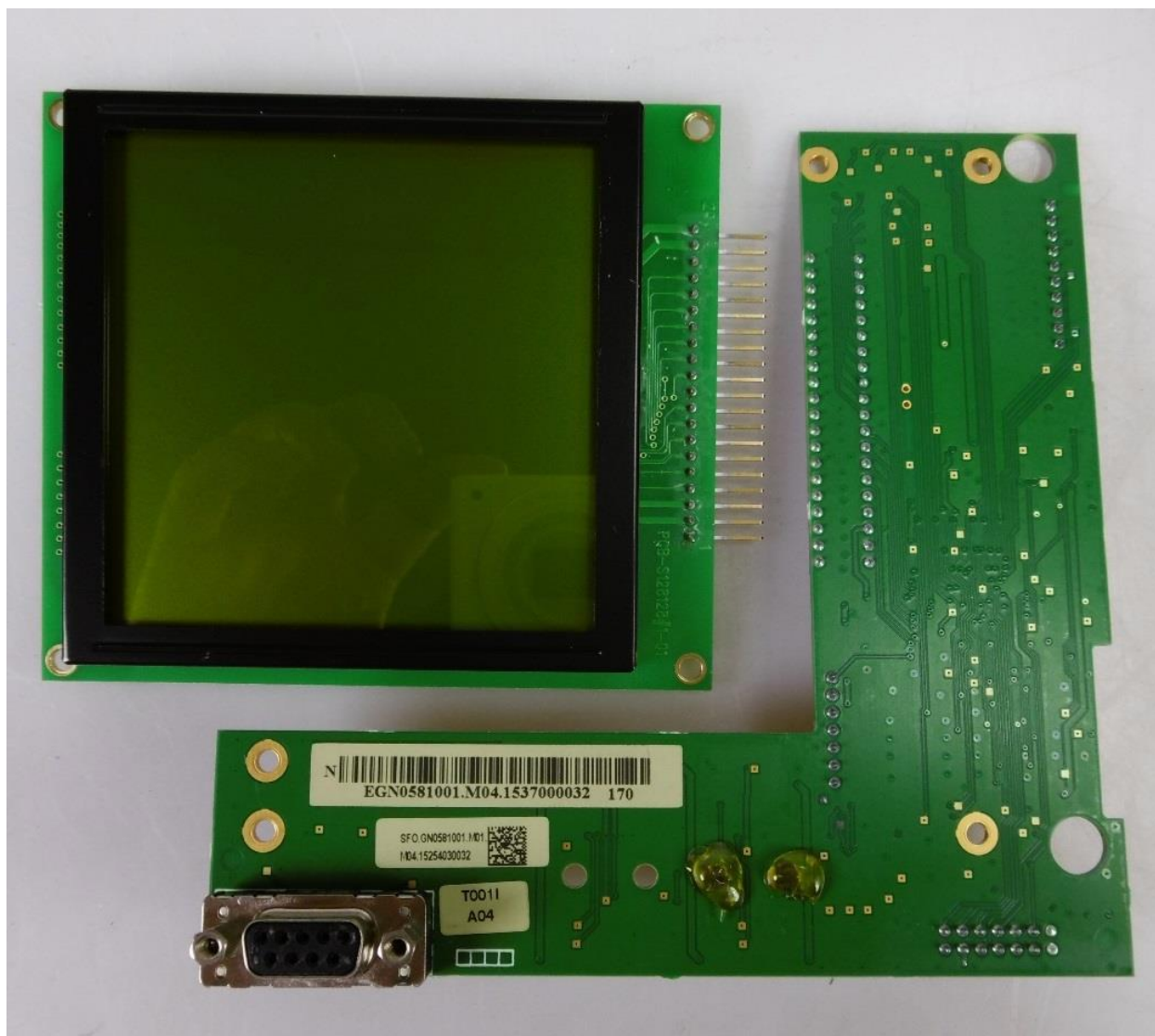
Display board and display/keyboard interface board (top view)
