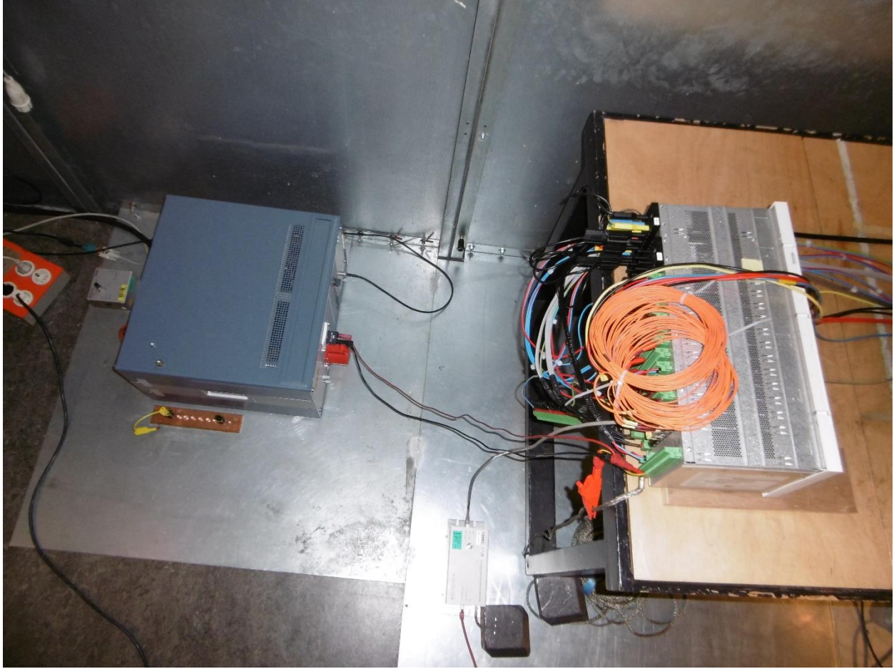
Conducted emission measurement on the power supply input port
