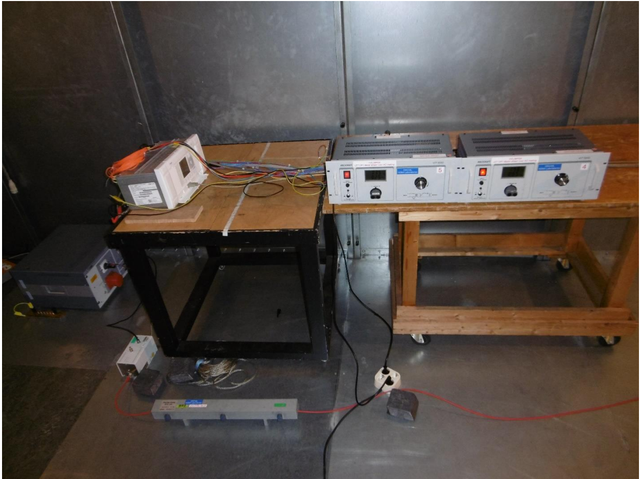
Conducted emission measurement on the LAN (RJ45) port
