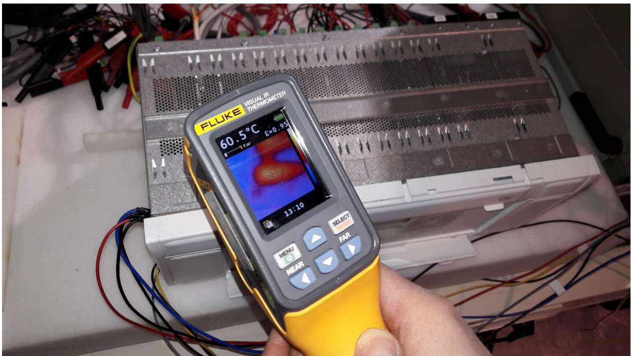
Enclosure temperature during the overload test.
