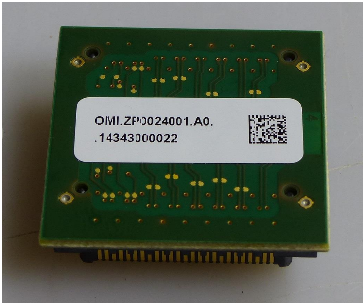
Connector board (bottom view)
