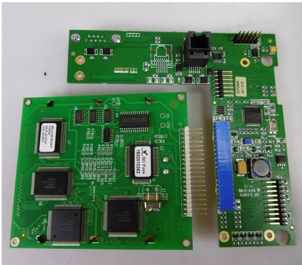
Display board and display/keyboard interface board (bottom view)
